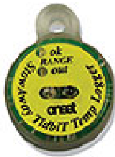
Figure 2.1 A StowAway Tidbit Temperature Logger as used to record sea temperature.
